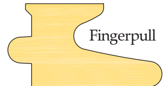
RWM 3042 \frac{7}{8} \times 1\text{-}\frac{5}{8} Fingerpull
