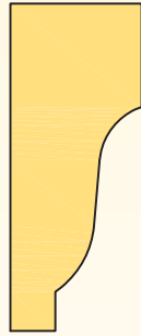
RWM 191 5/8 x 1-9/16 Shingle Mould
